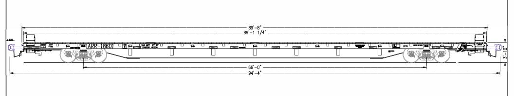
BUILT BY: EBENZER RAILCAR SERVICES, INC DATE BUILT: 2020 PURCHASED FROM: ERS, INC PLACED IN SERVICE: 2020 WHEELS: 36 INCH **BEARINGS:** 6½ X 9 AMERICAN HYDRAULICS, AMSTED 15" UNDERFRAME: AMERICAN HYDRAULICS, AMSTED FLOATING YOKES: AIRBRAKES: WABTECH ABDX-L HANDBRAKE: AAR RULE 13, GROUP U SIDE MOUNT LIGHTWEIGHT - LBS.: 81,500 CAPACITY - LBS.: 204,500
