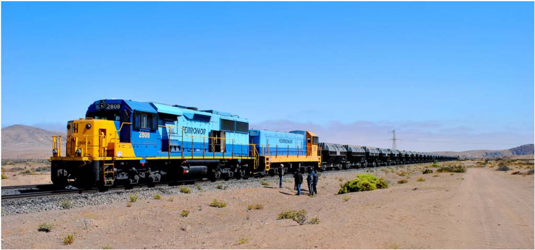
IRON ORE FERRONOR TRAIN 2808 LOCOMOTIVE EMD SD-49 CU M (EX GP-49 ALASKA RAIL) WITH DAUGHTER 288(WITHOUT DIESEL ENGINE WORK TOGETHER 2808) METER GAUGE TRACK (CHILE-VALLÉNAR)
